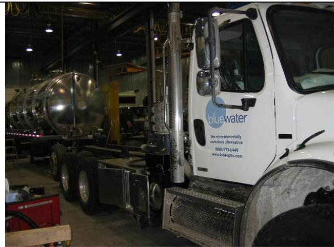
bluewater™ Recycler Truck chassis and cab
